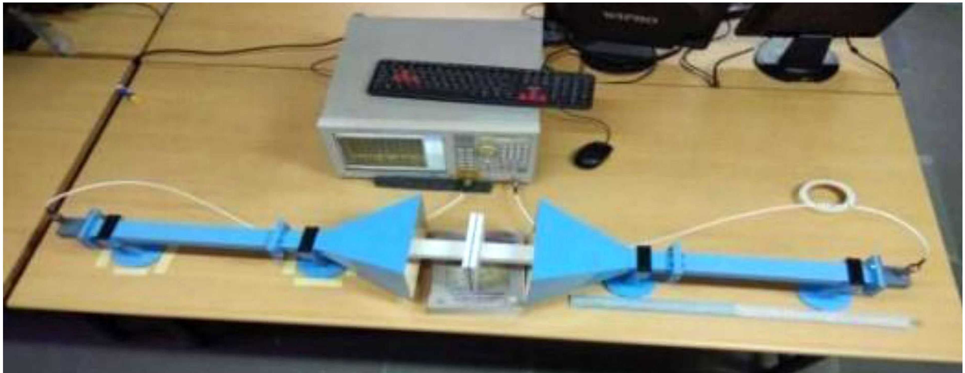
Photograph of WR-187 RDWG system for 3.95 to 5.85 Ghz frequency rang
