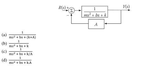
14. The closed-loop transfer function for the system is,
